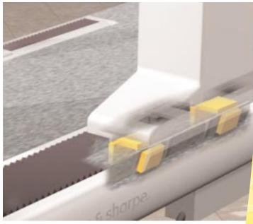
Wrap-around air bearings provide optimum measuring repeatability and long term system stability. Easy-maintenance, pre-loaded Belleville springs assure constant force over the machine's entire travel distance.
