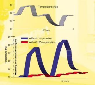
Temperature compensation systems have a dramatic effect on measuring machine accuracy. This chart illustrates how optional GLOBAL ACTIV structural compensation can significantly improve machine performance in fluctuating ambient temperature conditions.
