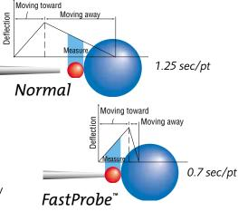
The result is a 50 percent increase in probe velocity, a smooth, continuous probe path between points, more precise data collection, and a significant increase in machine throughput.
